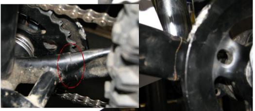
On the other handed, Matt "Abbot Be Mex" cracked the head tube on his hard tail during a Tuesday night ride in Lynn. Pedal-kicking a small gap, we all heard a snapping sound that even made Matt say..."what as that"! At first we though this noise was just sound resonating through the down tube...of course, the bike is only 3 months old. Upon further inspection, we noticed the head tube had a half-inch crack and was ovalized. Another bike slated for the recycling yard.
