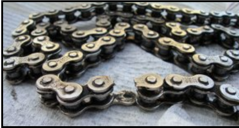
Figure 3.4 – Chain Stretch Leading to Link Assembly Failure.
