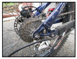
investing in a cassette removal tool for maintaining this drive-train component. In the end you will be able to clean the cassette more frequently in much less time then leaving it mounted on the hub. Again, there is no specific science for checking cassette wear but there are a number of techniques. We would suggest you consult a well qualified bicycle mechanic for assistance on identifying cassette sprocket wear.
