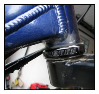
Once the bracket cups are threaded more then half way into the frame, they should begin to become snug and not to have any side-to-side play or looseness in the direction of the thread. If you thread the cups into the frame and they are loose, you may have a problem with the frame shell or bottom bracket cups. We would suggest taking your bike to a well qualified bicycle mechanic who can measure the bracket shell and bracket cups to ensure they are within manufacturers specifications.
