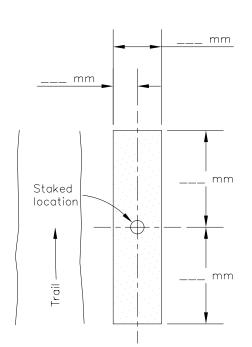
Placement tolerance within shaded area for avoiding obstacles.
